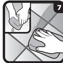
7 Wait for firm joints Lightly clean off excess grout with sponge. CAUTION: Do Not Over Water.
